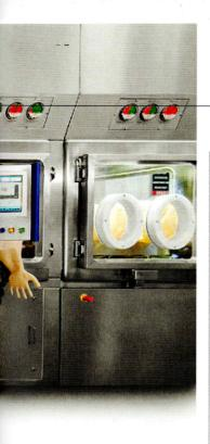
can also be classified as open RABS with airflow overspill to an ISO 7 or ISO 5 background, or closed RABS including closed ducted systems. They are also classified according to a leak rate.
